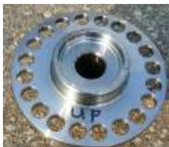
After drilling & front chamfering
