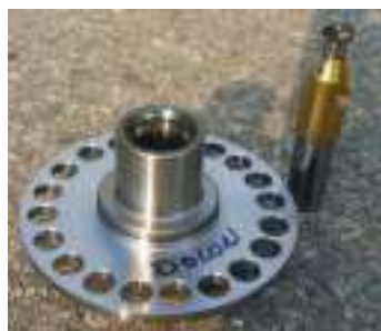
After drilling & back chamfering
