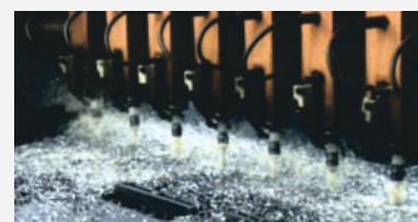
12 spindles machining feature used KRUZ body & IDPK inserts
